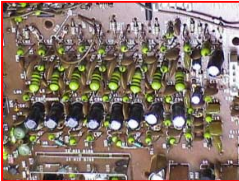
RF Board - Close up of band select filters (metal shield removed).
