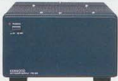
PS-53 Heavy Duty Power Supply(22.5A DC) Designed to match the TS-450S/690S. Supplies regulated 13.8V DC at 20.5 A with built-in cooling fan and protection circuits for maximum reliability.
