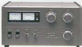
TL-992/TL-922A (for U.S.A) HF Liner Amplifier The TL-922/TL-922A are class AB 2 grounded-grid linear amplifiers developed by Kenwood using two high-performance EIMAC 3-500Z power tubes. They cover all bands 160 m through 10m (except the three new Amateur bands) for SSB, CW and RTTY modes of operation. (not usable with full break-in, semi break-in only)
