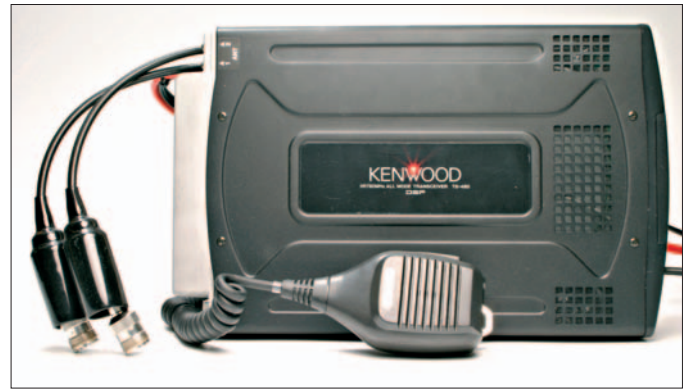
Fig. 2: Top view of the main transceiver unit, showing 'flying lead' antenna connectors (see text).
