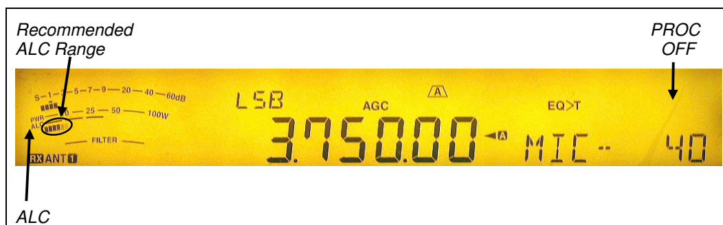
Figure 16: Setting up the microphone gain and ALC for unprocessed audio. The legend “MIC” appears on the display, and the legend “PROC” is absent. (The “RX” antenna happens to be enabled on this display, but this is not relevant to setting up the audio)
