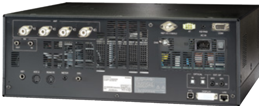
Figure 5 — The TS-990S rear panel showing the available connections.
