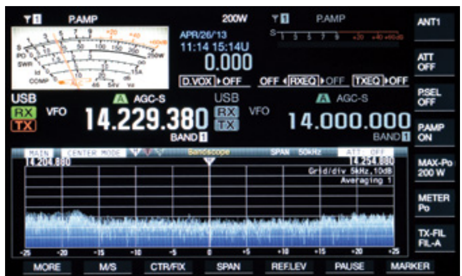
Figure 1 — The larger of the two colorful LCD panels can be configured to show many different operating parameters.
