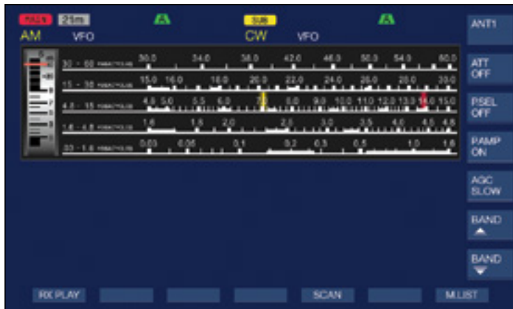
Figure 7 — Here's something I've not seen before. In the SWL mode, the top half of the TS-990S main display replicates a 1960s vintage Trio/Kenwood shortwave receiver.
