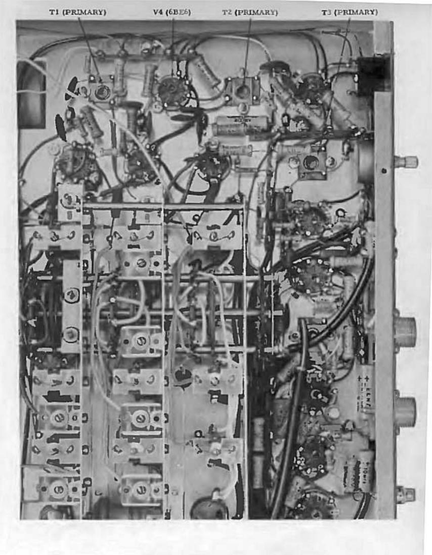
FIGURE B - UNDERSIDE ADJUSTMENTS
