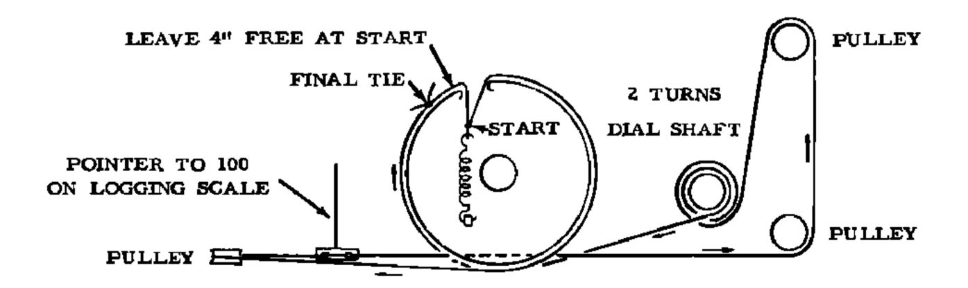
BANDSPREAD PULLEY FULLY COUNTER-CLOCKWISE.
