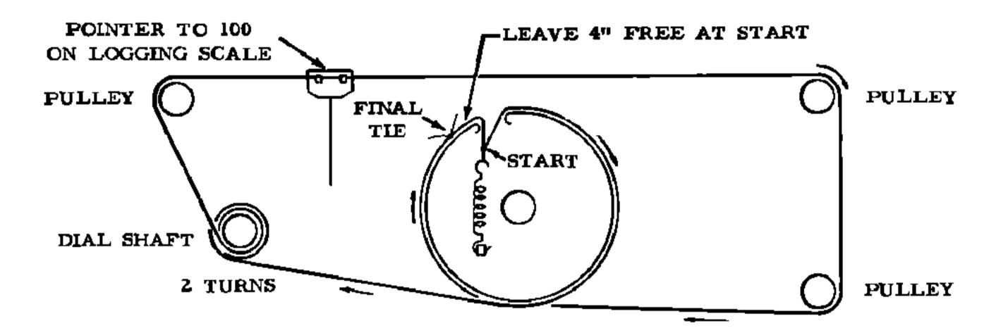
MAIN TUNING PULLEY FULLY COUNTER-CLOCKWISE.
