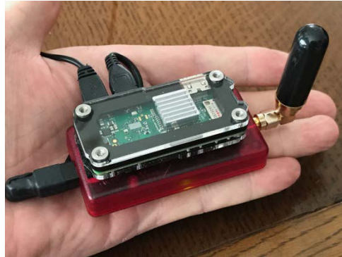
Lower Red case is DVAP, the upper is Raspberry Pi Zero W
