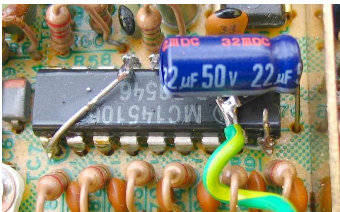
Fig 2 : side of MC145106 from pin 10 to 18
