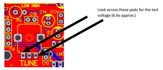
Once you're happy fit the tuning control which is a 10K potentiometer, there are two potentiometers in the kit but they are NOT the same, on the back of them (the bottom) you will see a marking, it will say either B1-03 or B1-02, we need the B1-03. Solder in place and also solder the two mounting lugs to hold the control on the PCB.
