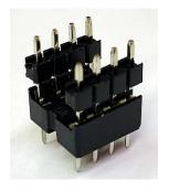
Now drop the adapter board on top of the pins. Take care and solder each pin to the adapter board. Now you can treat the assembly the same as a standard chip. Make sure that the 'chip' is plugged into the socket the right way round, if you look at the top of the chips board you will see the printed
