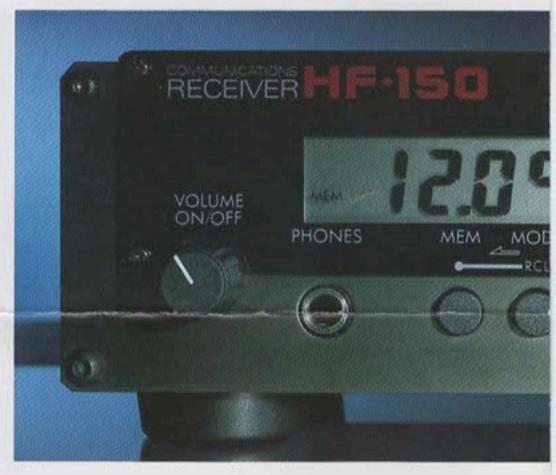
Reception modes are AM, Upper Sideband (USB), Lower Sideband (LSB), which also allows reception of CW/RTTY/FAX, and also included is an all new phase locked AM system which allows selection of either synchronous lower sideband or synchronous upper sideband and synchronous
