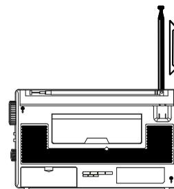
4. Press and hold the [∧] or [∨] buttons for at least a half second or more and the radio will scan all the frequencies in that band, and will stop automatically each time it lands on an active station. Signal strength is recorded on the SIGNAL STRENGTH INDICATOR.
