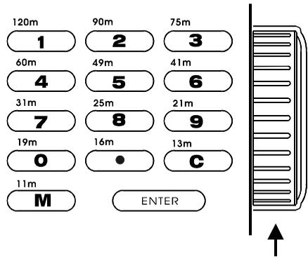
8. Rotate the BFO PITCH control to adjust the signal quality.
