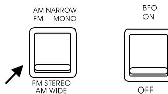
If you plan to listen to Morse code, referred to as CW (continuous wave), set the BFO switch to ON position. If you encounter too much noise as you tune, set the AM NARROW/WIDE switch to NARROW position.
