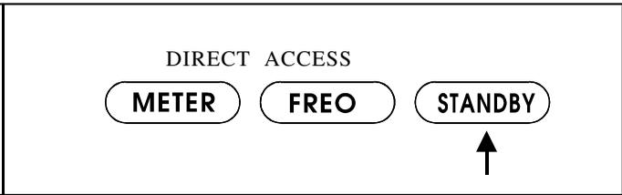
5. You may select radio or buzzer alarm to wake you by setting STANDBY:BUZZER/RADIO selector switch.
