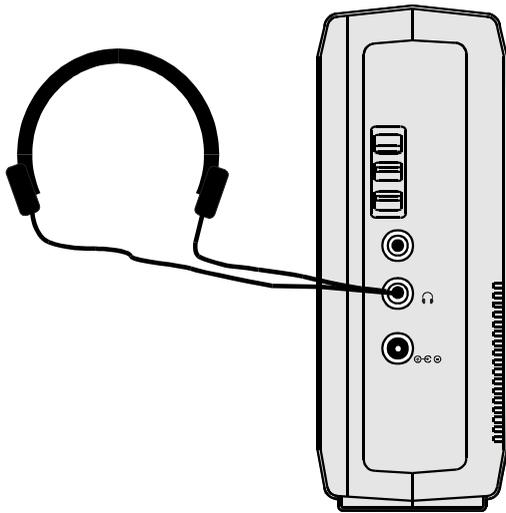
Because the radio is capable of receiving FM multiplex stereo, Stereo HEADPHONES Should be used. When listening to stereo FM, be sure that the FM: STEREO/MONO switch is set to the STEREO position.
