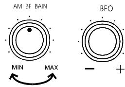
9. Reduce strong signals by using the RF GAIN control. This also reduces interference and noise.
