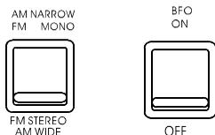
Many stations transmit voice signals with a suppressed carrier in the *single side band*. (SSB), part of the radio transmission spectrum that lies to the side of the primary frequency signal. Many amateurs who operate transmit below 10 Mhz generally use the *lower side band* (LSB). Above 10 MHz, they usually use the *upper side band* (USB). Commercial utility stations generally use the USB. A carrier has to be added to make these signals audible.
