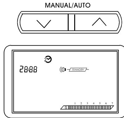
5. Press and hold the [∧] or [∨] buttons again to resume scanning. When you reach the upper or lower limits of the band, the scanning starts all over again as long as the button is depressed once more.
