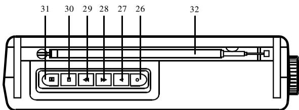
1. To Fast-Forward the tape, press FAST-FORWARD [29].
