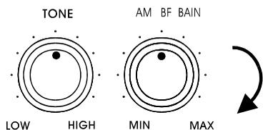
If you encounter interference, adjust the control in both directions until you obtain the best compromise between your station and the interference.
