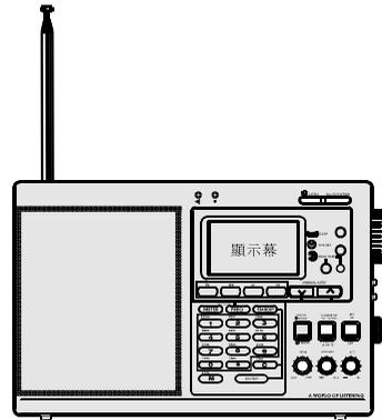
3. Set the BFO switch to the ON position.
