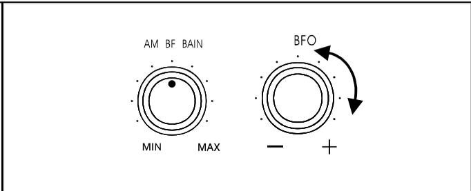
9. Rotate the RF CAIN control to dampen strong signals. This can improve signal clarity as well.
