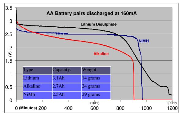
The above graph shows the discharge rates of the typical battery options. It shows that the single use Lithium and 2500mAh NiMh can significantly outperform even the best alkaline batteries. New low self discharge offerings like the Panasonic "Eneloop" or Eveready "Recharge Extreme" can be considered if you use the sniffer regularly and wish to save money in the long run.
