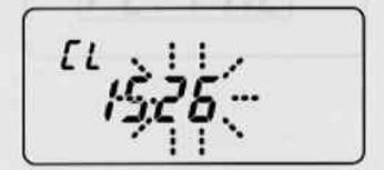
6 Set the clock to the current minute by turning the DIAL knob 8.
