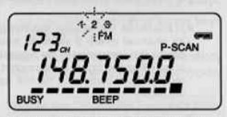
To cancel, repeat steps 1 and 2. Channel memory reading starts in the channel being received or scanned.
