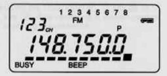
To cancel the program registered, select it through program scanning and perform steps 2 and 3 (when all registered programs are deleted or all the programs for the specified bank are deleted, a beep is sounded and the receiver enters memory read status in the channel deleted last).
