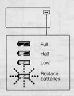
Display shows nothing when the batteries completely discharge.
