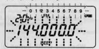
3 Enter the lower limit of the frequency range with the numeric keys.
