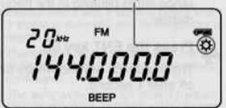
To turn off the lamp, press the LAMP button ③. The lamp and mark [☼] are turned off.
