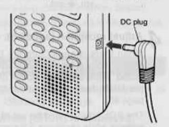
2 Plug the AC adaptor into an AC outlet; or plug the cigarette lighter plug into the cigarette lighter socket (12VDC).
