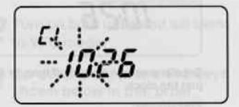
4 Set the clock to the current hour by turning the DIAL knob 8.
