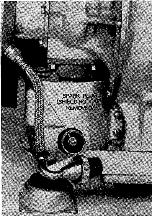
FIGURE 4.—Spark plug and baffle—Continued.
