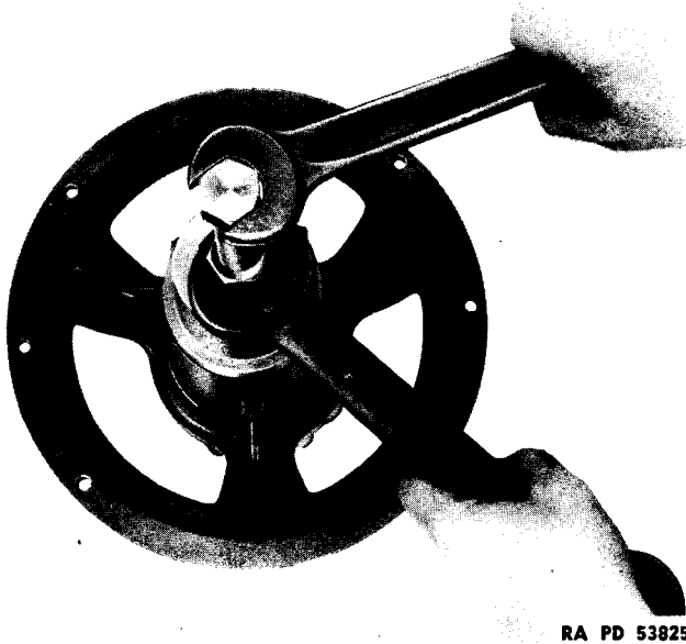
Figure 26 — Assembling Crankshaft, Using Fixture HL-AA-205 (2)
