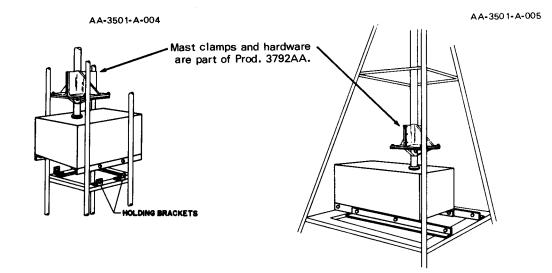
4. On top of large towers. Where a large, flat-topped tower is available, the rotator may be installed directly on top. This may be secured by bolting directly and securing the four corners with four angles supports to the legs of the tower as shown in the illustration.
