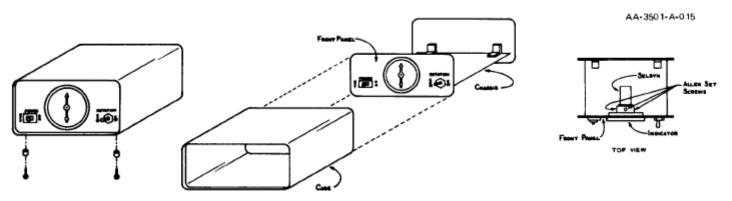
The indicator dial will usually require slight adjustment for accurate readings. Remove the chassis as shown above. Loosen the three Allen screws in the dial frame holding the selsyn and carefully rotate the selsyn in the frame until the dial indicates the proper direction. Tighten the Allen screws and replace the cabinet. *CAUTION*
