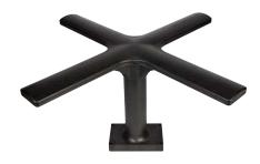
This L3Harris vehicular X-wing antenna is a bolt-on, dual-mode antenna designed for On-The-Move operations. This ruggedized, low-profile solution provides 50 watts maximum power with a high-angle circular polarized SATCOM mode and low-angle linear polarized mode for Line-Of-Sight. Two connector ports are located on the bottom of the antenna, type N female for high-angle and TNC (F) for low-angle. No antenna assembly is required, supporting rapidly deployed connectivity.
