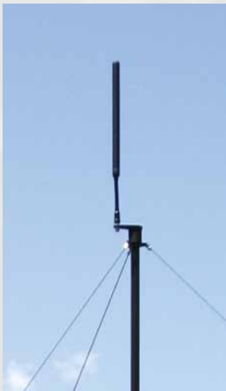
Model 3505, 225-1000MHz manportable antenna mounted on MA-703
