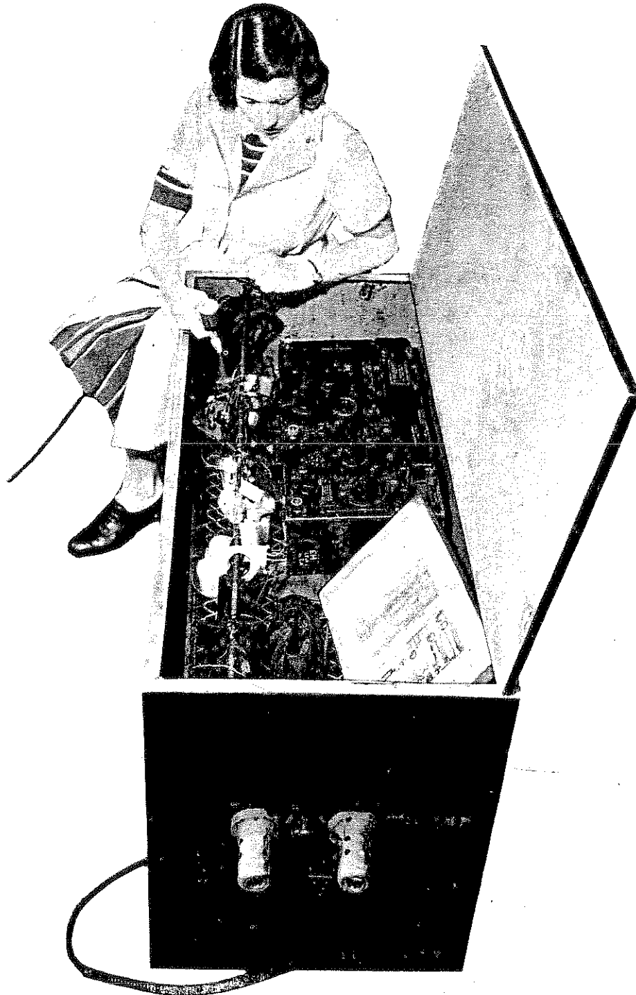
FIGURE 5—Spraying mould test chamber with mixed spores.
