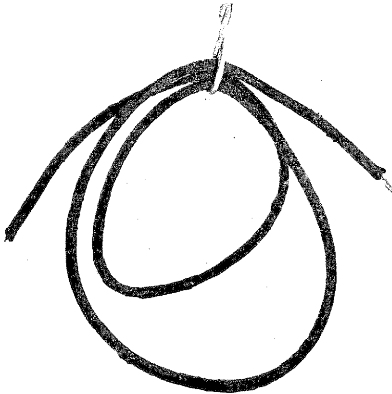
FIGURE 9—Mould on lacquered cotton-covered hook-up wire.
