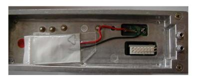
Solder the battery wires as shown above. Ensure that the –ve battery terminal is connected so as to bridge the solder bridge as without the bridge being in place, battery backup is not enabled.
