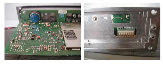
The above illustrates a radio with memory backup battery fitted
