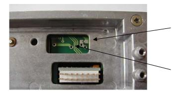
Identify the Battery connections on the radio, and also the solder bridge that will need to be bridged with solder as shown in the photo above.
