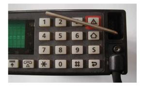
Flip up the handle and remove the code plug if one is fitted to gain access to the allen screw behind.
