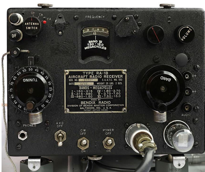
Figure 3. RA-1B front panel (refurbished radio)
