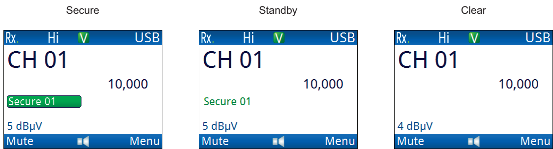
Figure 65: Channel screen showing transmit/receive status for CES-128 voice encryption
