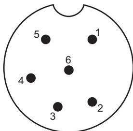
Table 37: Pinouts of the antenna control connector on the RF unit
