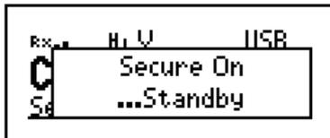
If you are in the Channel List, the CES-128 voice encryptor in standby mode is indicated by the text **Secure <index>[P]** underlined at the bottom left of the channel screen. For example:
