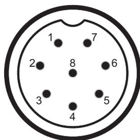
Table 36: Pinouts of the CIB connector on the RF unit (NGT AR and SR Transceivers only)
