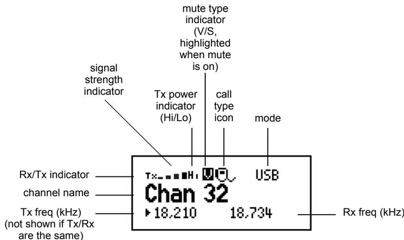
If the transmit and receive frequencies are the same, the frequency is only displayed in the receive frequency position on the right side of the screen, and the Rx indicator arrow is not used. The Rx/Tx indicator shows whether the transceiver is receiving or transmitting.
