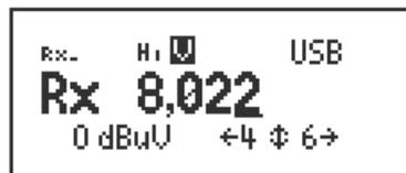
If you are able to transmit during Free Tune, the Rx is replaced by a Tx within the amateur band frequencies, as shown below. For information on amateur band frequencies see [Table 32 on page 288](#).
