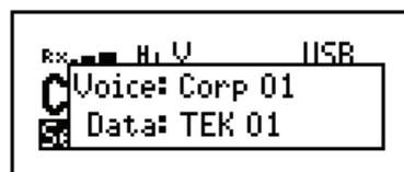
If you are in the Channel List, the active AES-256 digital data encryptor is indicated by the text **TEK <index> Dat** at the bottom left of the channel screen. The active CES-128 voice encryptor is indicated by the text **Secure <index>[P]** highlighted at the bottom left of the channel screen. These screens alternate. For example:
