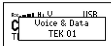
If you are in the Channel List, the active AES-256 digital voice encryptor is indicated by the text **TEK <index> <1k2|2k4>** at the bottom left of the channel screen. For example:
