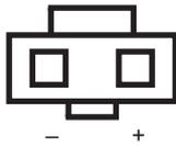
Table 39: Pinouts of the fan connector on the RF unit
