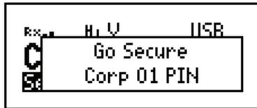
If you are in the Channel List, the active CES-128 voice encryptor is indicated by the text **Secure <index>P** highlighted at the bottom left of the channel screen. For example:
