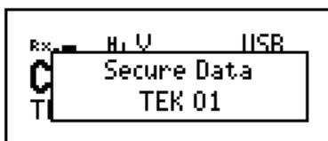
If you are in the Channel List, the active AES-256 digital data encryptor is indicated by the text **TEK <index> Dat** at the bottom left of the channel screen. For example:
