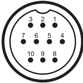
Table 40: Pinouts of the 10-way connector on the RF unit (NGT AR Voice and VR Transceivers only)
