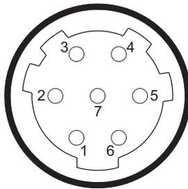
Table 42: Pinouts of the handset connector on the junction box (NGT *AR* and *SR* Transceivers only)
