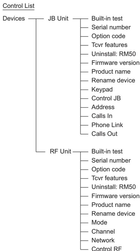
Figure 36: The Devices entry in the Control List (NGT AR Voice and VR Transceivers only)
