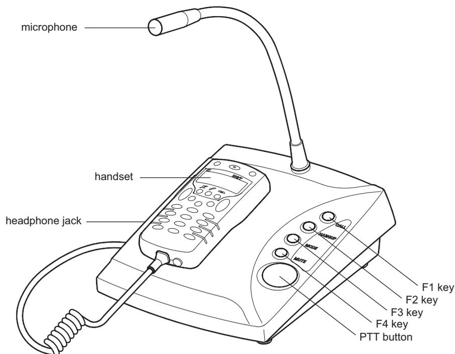
**NOTE** With a Code 766 Desk Console, the handset connects to the rear of the console.
