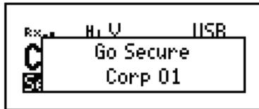
If you are in the Channel List, the active CES-128 voice encryptor is indicated by the text **Secure <index>** highlighted at the bottom left of the channel screen. For example:
