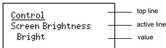
The handset screen also displays information screens such as the channel screen in the Channel List, and the time screen in the Control List.
