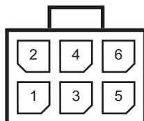
Table 41: Pinouts of the 6-way connector on the RF unit (NGT AR Voice Transceivers only)
