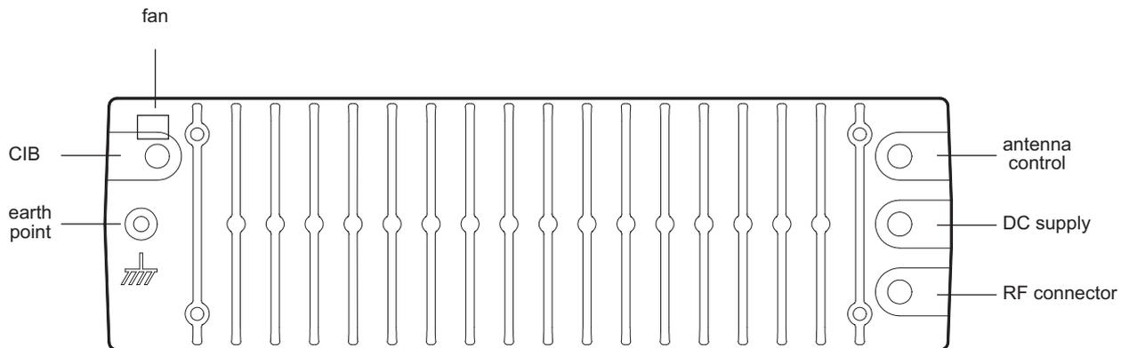
Figure 43: Back panel of the 2011 RF Unit (NGT *AR Voice* and *VR* Transceivers only)
