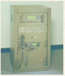
Military RT7000-based rack system with telephone interface and encryption.
