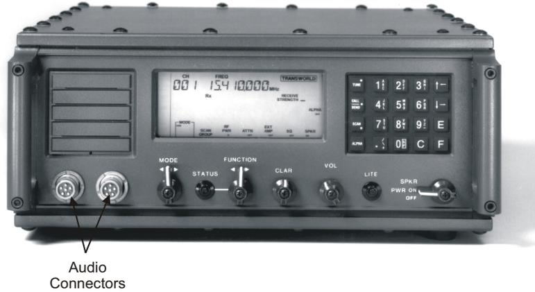
**Figure 2-1. Front Panel Connections**
