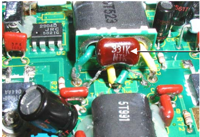
Fig.1 C27, 330 pF on 05P0667 with 2SC2879A
