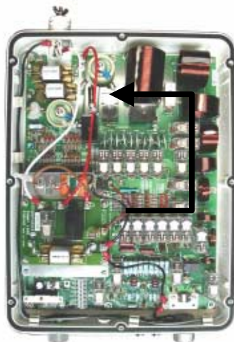
Fig.6.2.2 Order of relay test
