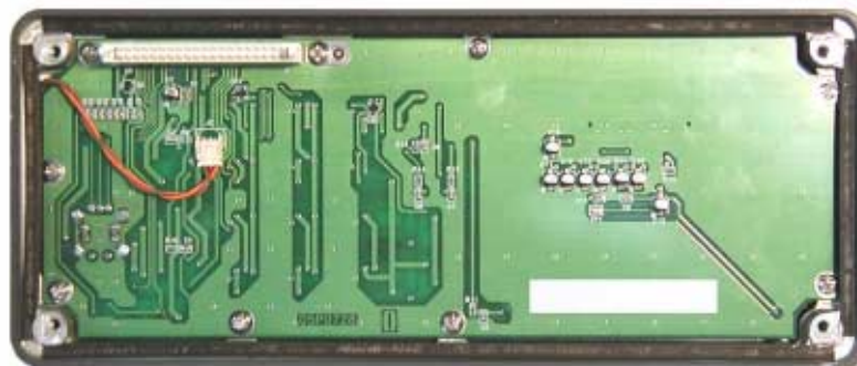
Fig.2.1.9 PANEL board (05P0728), side - Display unit with shield cover removed
