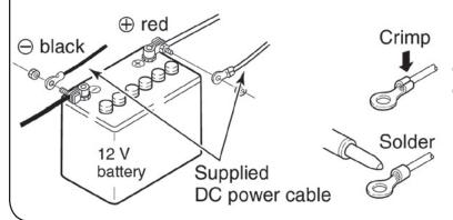
Make sure the back up battery is correctly connected. Use a cable with following current capacity. Solder or clamp the cable plug when connecting the power cable to the backup battery to prevent voltage drops.
