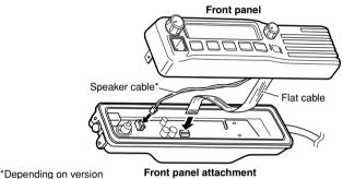
③ Screw the 3 supplied bolts to attach the front panel and the attachment.
