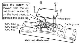
(5) Connect the supplied flat cable\* and ground cable (coming from the RMK-2) as shown below.
