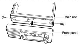
⑤ Unscrew the 4 screws, then remove the rear plates from both the front panel and main unit attachments.
