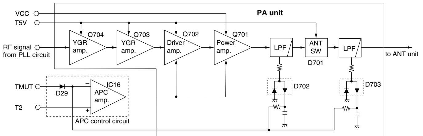
(MAIN unit; IC16; pin 3), and the "T2" signal from the D/A converter (MAIN unit; IC12, pin 23), controlled by the CPU (MAIN unit; IC22), is applied to the other input for reference. When antenna impedance is mismatched, the detected voltage exceeds the power setting voltage. Then the output voltage of the differential amplifier (MAIN unit; IC16, pin 4) controls the input current of the drive (PA unit; Q702) and power (PA unit; Q701) amplifiers to reduce the output power.
