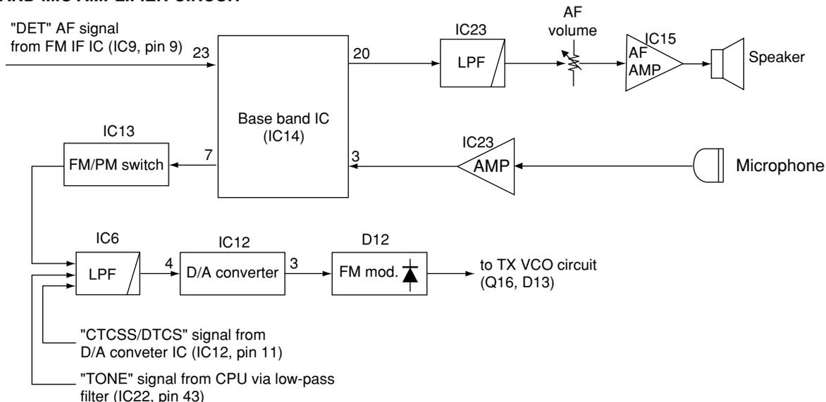
posed of microphone amplifier, compressor, scrambler, limiter, splatter filter, MSK modulator, etc. at the microphone amplifier section.
