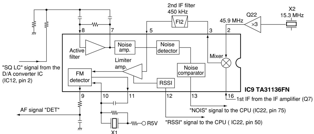
The 2nd IF signal from the 2nd mixer (IC9, pin 3) passes through the ceramic filter (FI2) to remove unwanted heterodyned frequencies. It is then amplified at the limiter amplifier section (IC9, pin 5) and applied to the quadrature detector section (IC9, pins 10, 11) to demodulate the 2nd IF signal into AF signals.
