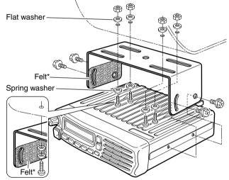
When using self-tapping screws
