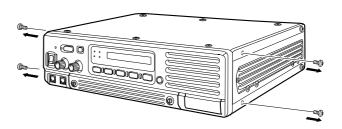
6 Attach the MB-78 to the top side of the repeater. Then tighten the supplied screws (M4  $\times$  8) and 2 screws removed from each side of the repeater. (6 screws in total)
