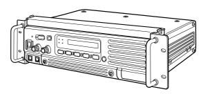
Turn the repeater upside down, and remove the 4 legs before mounting into the 19 inch rack.
