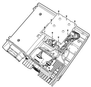
③ Cut the pattern on the PCB at the RX AF circuit (CP1) and TX mic circuit (CP2) on the LOGIC unit as shown at right.
