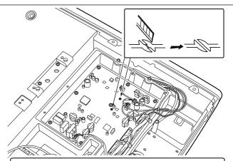
**NOTE:** Be sure to re-solder above disconnected points, otherwise no TX modulation or AF output is available when you remove the scrambler unit.
