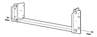
② Remove the handles from the bottom bar. And turn the handles upside down, then replace the handles right side and left side.
