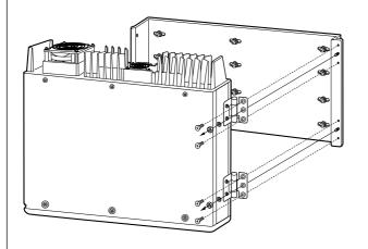
$\ensuremath{\mathfrak{G}}$  Tighten the 3 supplied screws (M5  $\times$  12) to the other side.
