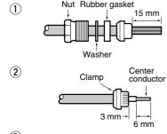
Slide the nut, flat washer, rubber gasket and clamp over the coaxial cable, then cut the end of the cable evenly.
