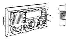
© Secure the assembly using the supplied mounting bolts and washers.
