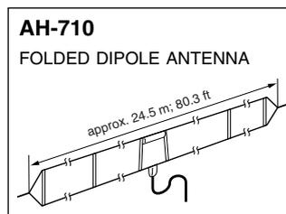
Covers from 1.9 to 30 MHz band. Has an SO-239 connector. Easy to assemble (non-kink construction).
