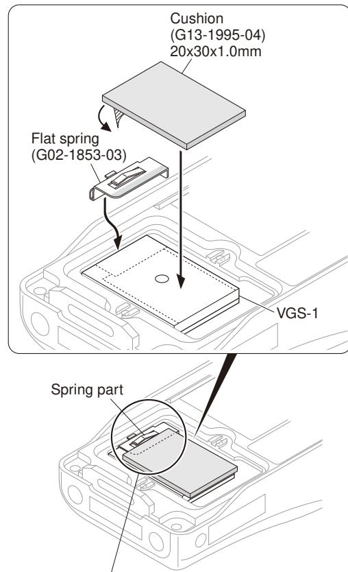
6. Insert the flat spring (G02-1853-03) between the VGS-1 and the chassis as shown in the figure.
