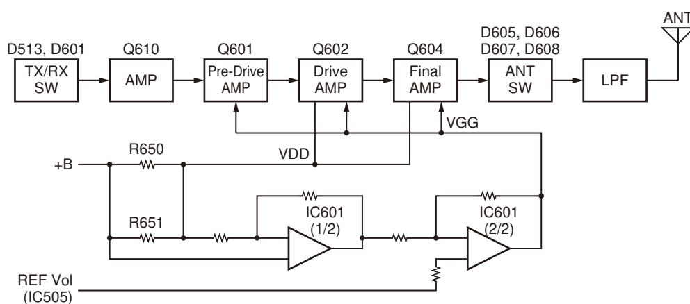
Fig. 6 Drive and final amplifier and APC circuit
