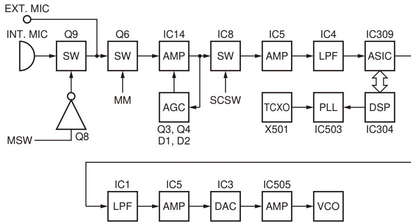
**Fig. 5** Audio band and Baseband circuit
