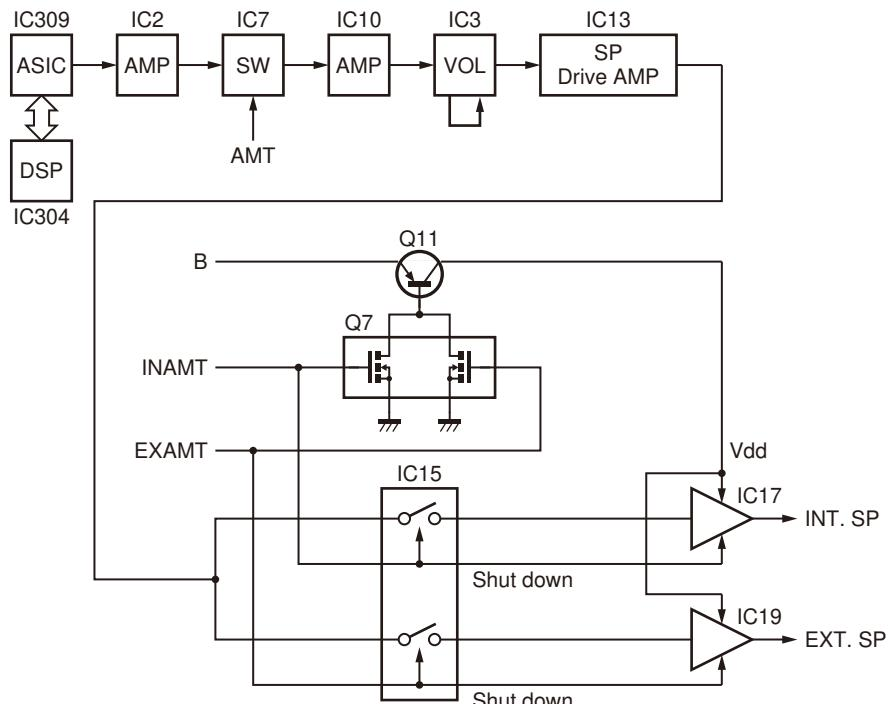
Fig. 3 Audio amplifier circuit
