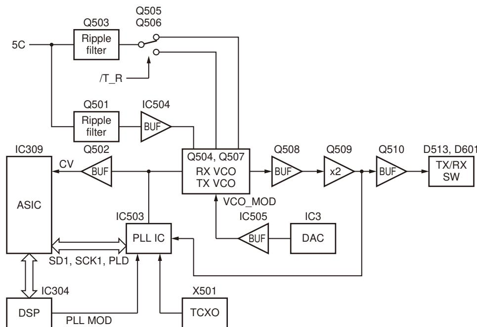
Fig. 7 PLL block diagram
