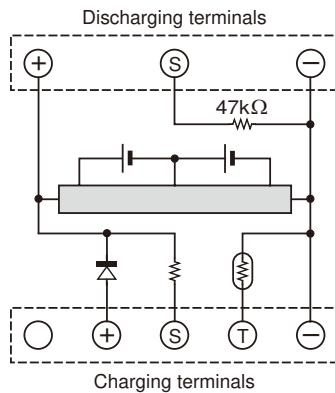
**KNB-54N (Ni-MH Battery Pack): 7.2V 2500mAh**
