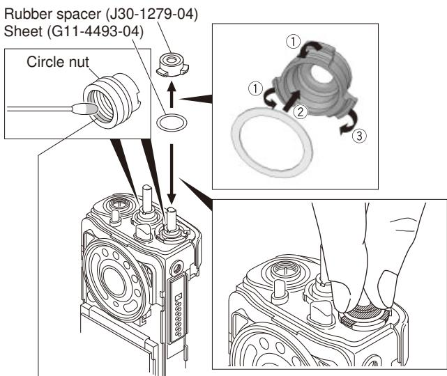
Apply the bond (W05-0019-00) or "THREE BOND 1401B" around the inside of the circle nut before tightening the circle nut.
