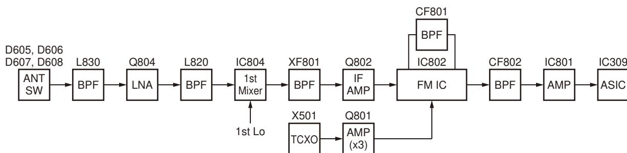
Fig. 2 RF and IF circuit
