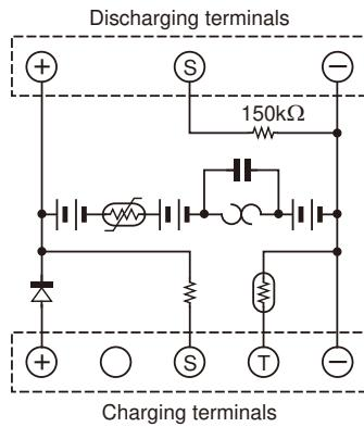
**KNB-33L (Li-ion Battery Pack): 7.4V 2000mAh**
