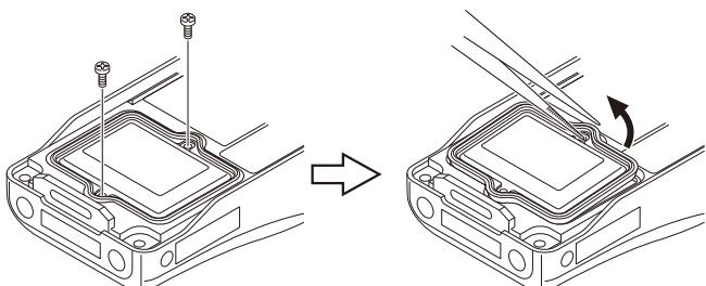
3. Remove the OPTION PCB from the connector (CN321) of the TX-RX PCB.
