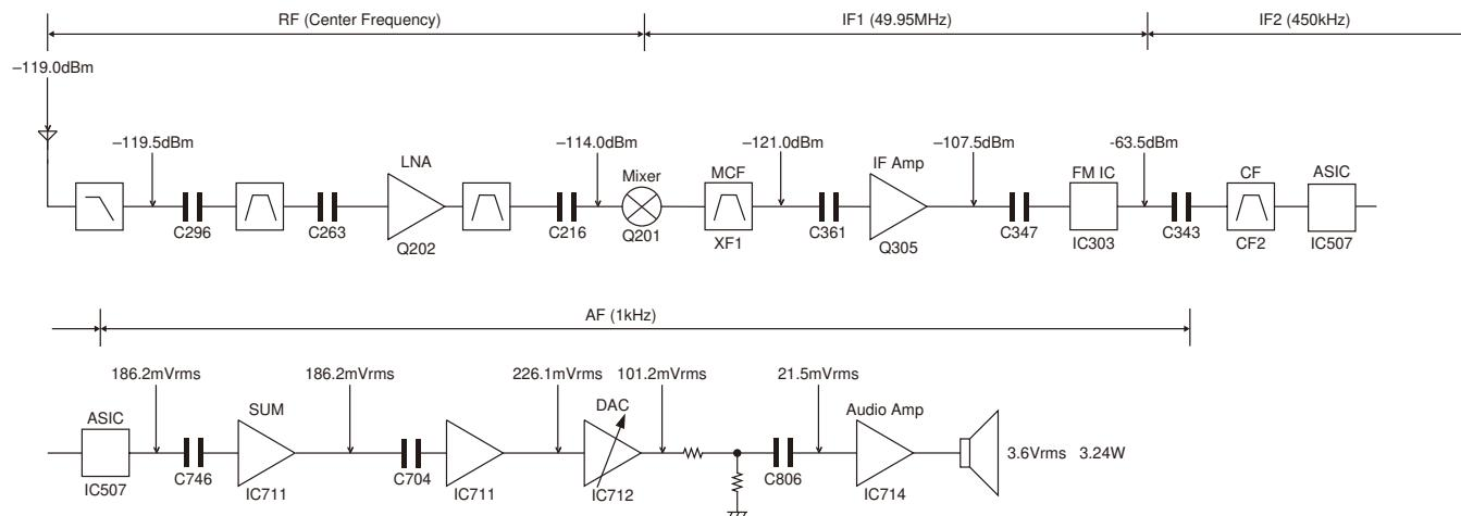
To make measurements in the AF section, connect the AC level meter. (ANT input:-53dBm, 1kHz FM, 3kHz DEV (Wide))
