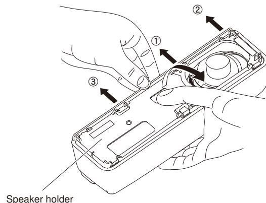
5. When removing the TX-RX PCB, first remove the top packing.
