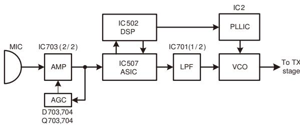
Fig. 4 Transmitter System
