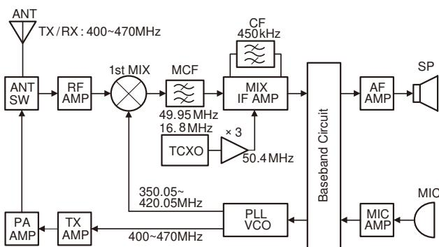
Fig.1 Frequency configuration
