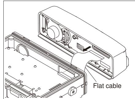
4. Hook the finger to hole and while pulling the speaker holder to this side, expand the panel side of ① to ③, and remove the speaker holder from the front panel.
