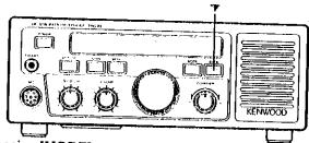
Pressing [MODE], pressing [DATA], or changing the channel after entering Data mode cancels Data mode.
