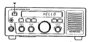
To switch OFF the radiotelephone, press [POWER] again.
