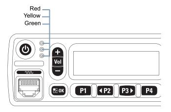
Blinking red – Radio is receiving an emergency transmission or has failed the self-test upon powering up, or has moved out of range if radio is configured with Auto-Range Transponder System.
