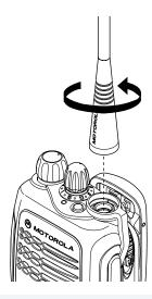
Turn the antenna counterclockwise to remove it.
