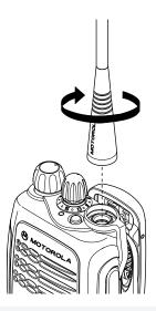
Turn the antenna clockwise to attach it.
