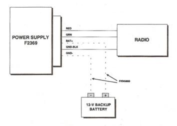
This power supply also serves as a charger for the external backup 12-V battery, if connected. When AC power failure occurs, the battery functions as the main power source. When AC power is again available, the power supply charges the battery.
