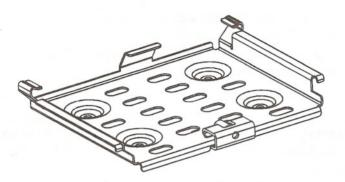
Step 2. Use the four supplied screws to fasten the mounting tray bracket to the bottom of the radio housing.
