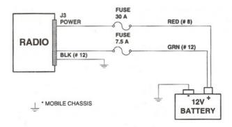
Step 1. Bring the power connector on the DC Power Cable to the radio DC connector but do not attach it to the radio. Then bring the three heavy wires (RED, GRN, BLK) to a 12-V battery, passing them through access holes as required.
