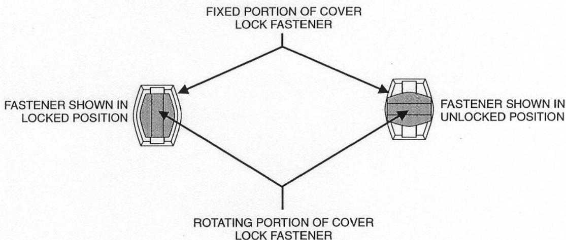
Figure 5. Oven Cover Lock Fastener
