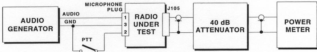
b. Transmitter Test Setup with Terminating Power Meter
