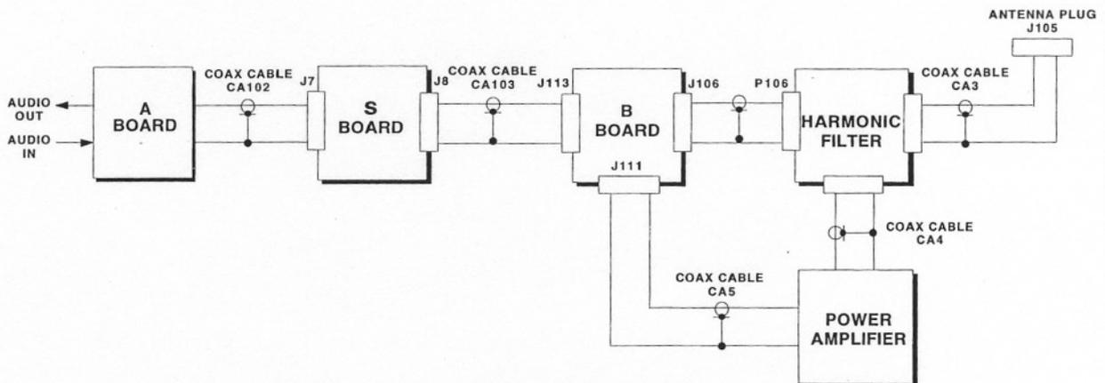
Figure 7. RF Connections between the Radio's Units
