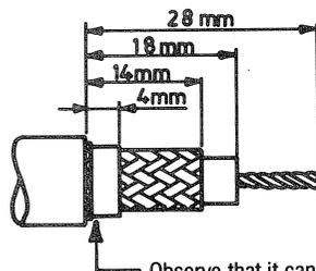
Observe that it can be necessary to isolate outer screen with insulating tape to ensure that it is not grounded.
