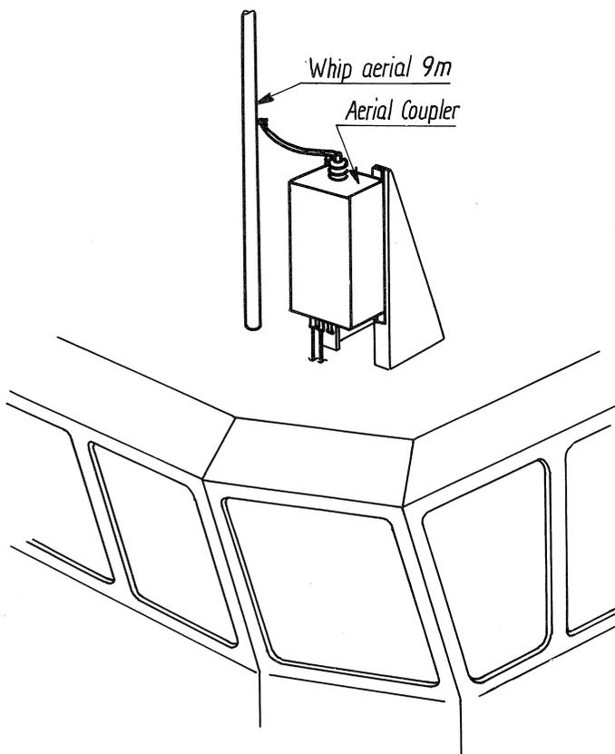
AT2110 has to be grounded through the two lower mounting holes.
