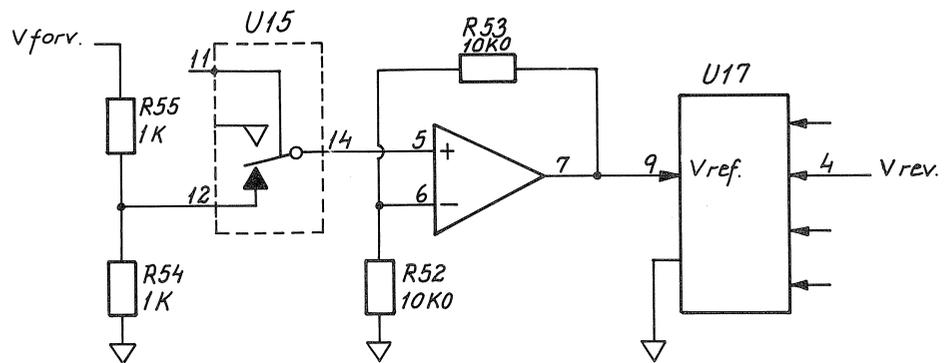
When measuring RHO the Vforward is connected to reference input of the ADC (U17, pin 9). Vreverse is connected to pin 4. The result of the ratiometric measuring is the parameter RHO, defined by Vreverse divided by Vforward.  $RHO = V_{reverse}/V_{forward}$ .
