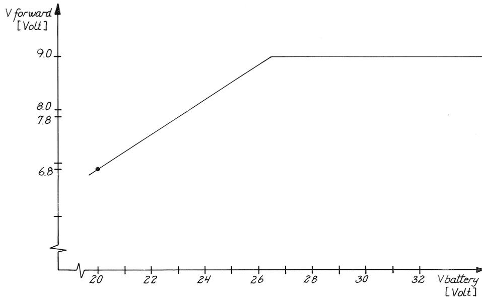
Fig. 2. Nominal values of the V<sub>battery</sub>, V<sub>forward</sub> maximum.
