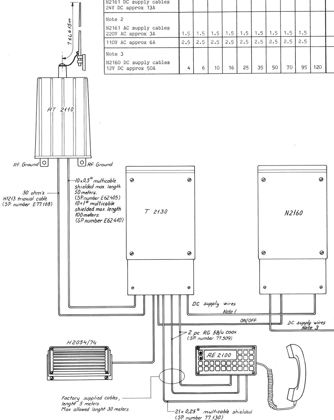
2.2.6. MAIN CABLE PLAN WHEN SUPPLIED FROM AC, USING N2161 AC TO 24V DC POWER SUPPLY.
