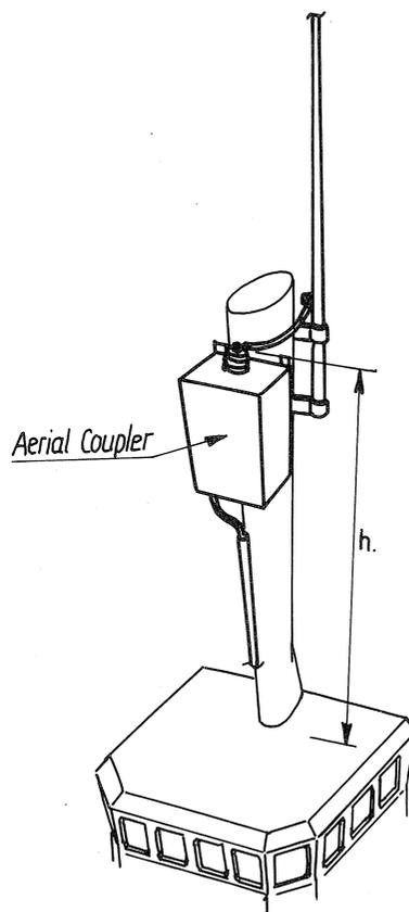
AT2110 has to be grounded to the mast if a metal mast.
