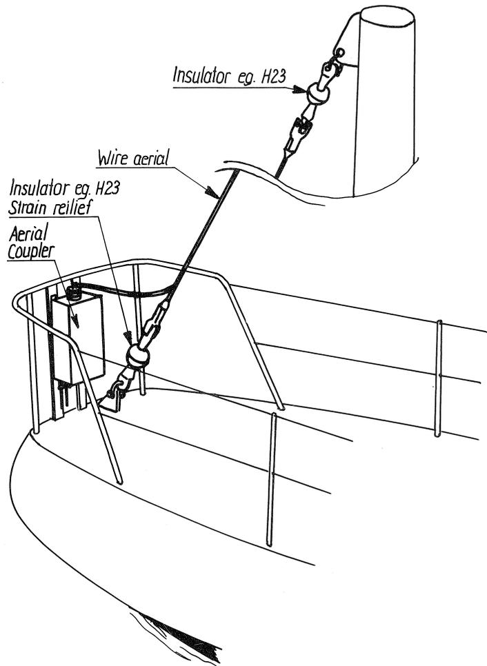
AT2110 has to be grounded e.g. to the handrail or other metal parts.
