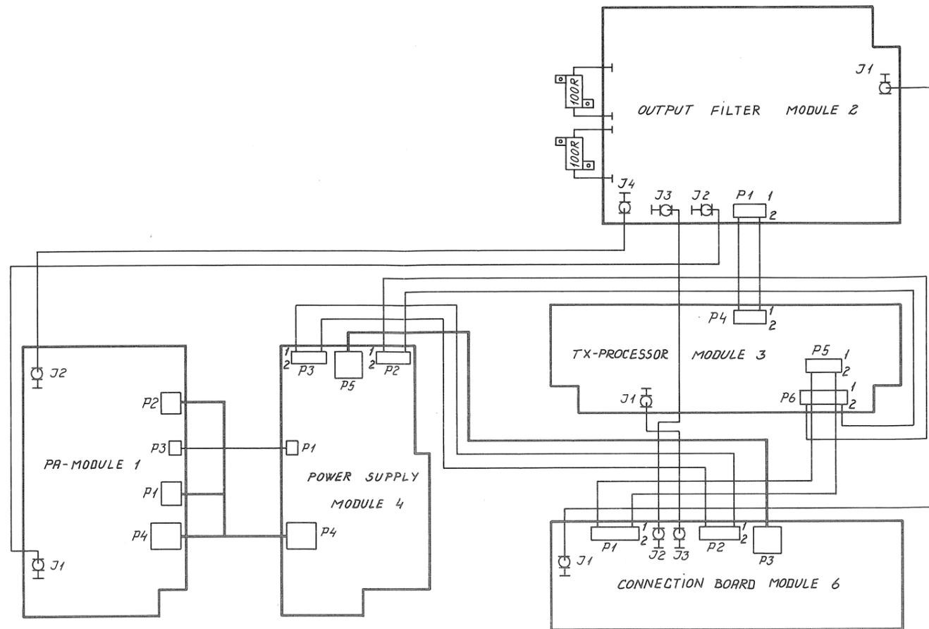
CABLE 1 : TX-PROCESSOR TO POWER SUPPLY I
