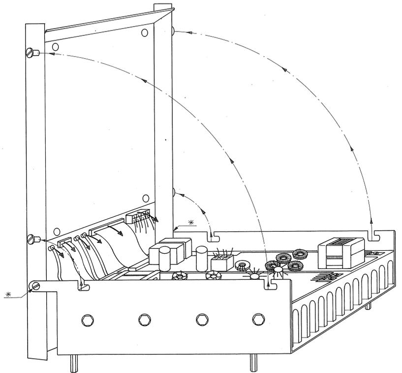
After disconnecting all cables on the connection board, remove the inner chassis by dismounting the 2 screws marked \*.
