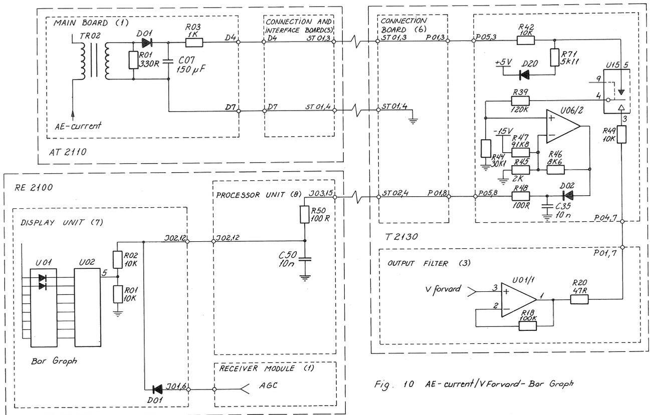
Fig. 10 AE-current/VForward - Bar Graph
