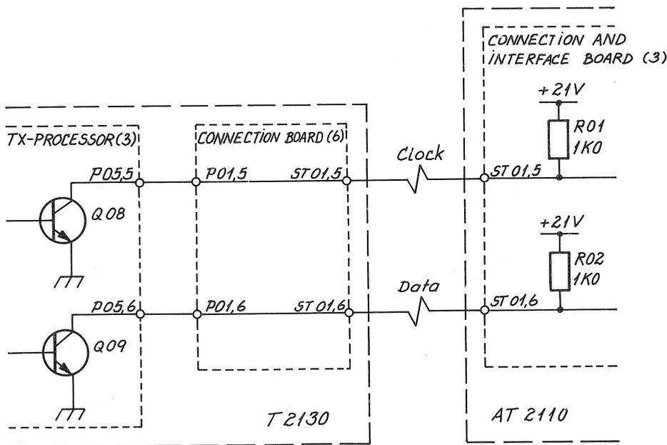
The clock and data lines between the T2130 and AT2110 are then held at a very low impedance which reduces the possibility for noise introducing unintentional clock and data pulses.
