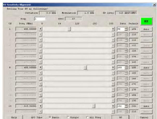
You may select the alignment type from the “Radio” button located at the bottom of the screen (ADJ Type), as needed.
