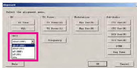
When perform the RX Tune and SQL alignment, the RF level shows this unit according to this setting.
