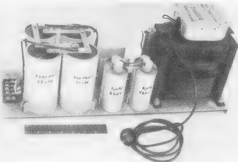
Power Supply — Typical 240 V to 24 VDC. Note — rule in foreground is seven inches long.
