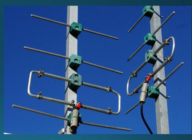
Two inexpensive 2M Yagis, like Cushcraft 124WB, work great as a Satellite array. Then, for VHF Contests, stack 'em normally and use the same phasing cables!
