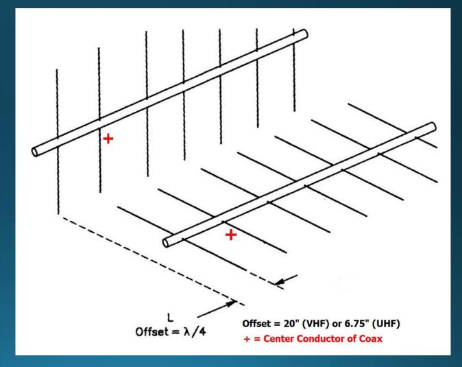
When installing a vertical or cross-polarized beam:
