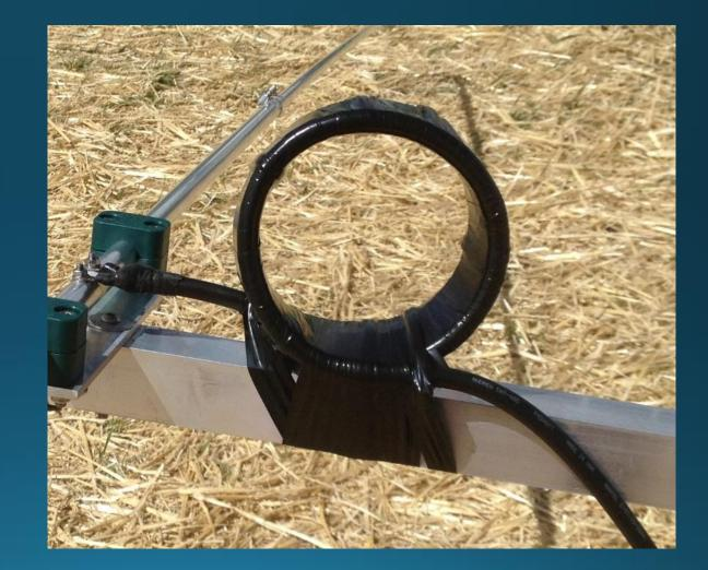
Use the minimum possible length of pigtails from Balun; apart of the driven element total length!
