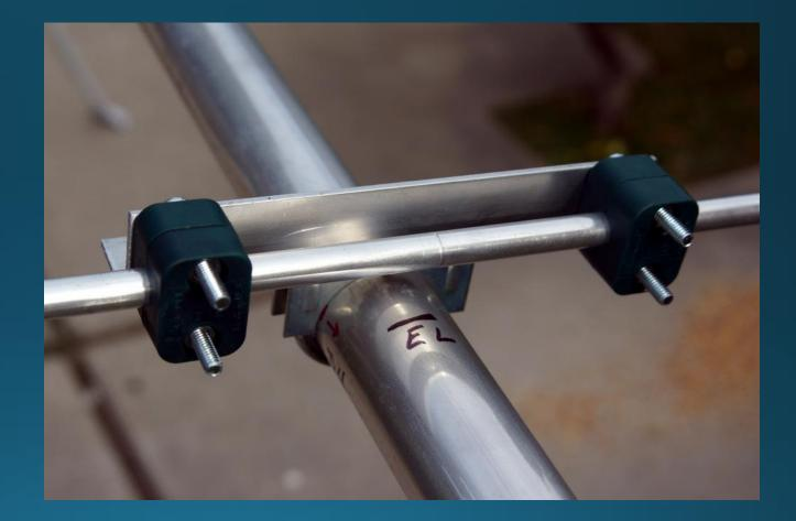
Larger "Guillotine" U-bolts will hold larger elements for 10-15 meters stoutly in place on 3" boom.
