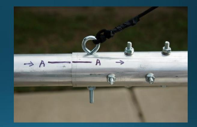
An inner sleeve, carefully cleaned and drilled, makes a very sound splice. Additional sleeves or a hardwood dowel may be further inserted to strengthen the joint. Lubricate everything!
