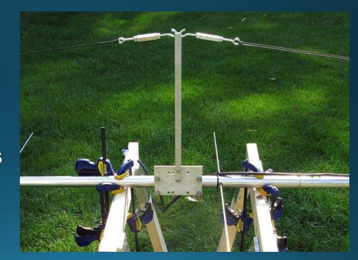
Eye bolt fitted to boom serves as attachment point for top support.
