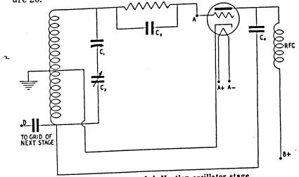
FIGURE 26. Shunt fed, Hartley oscillator stage.
