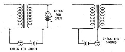
FIGURE 9. Testing transformer with continuity indicator.
