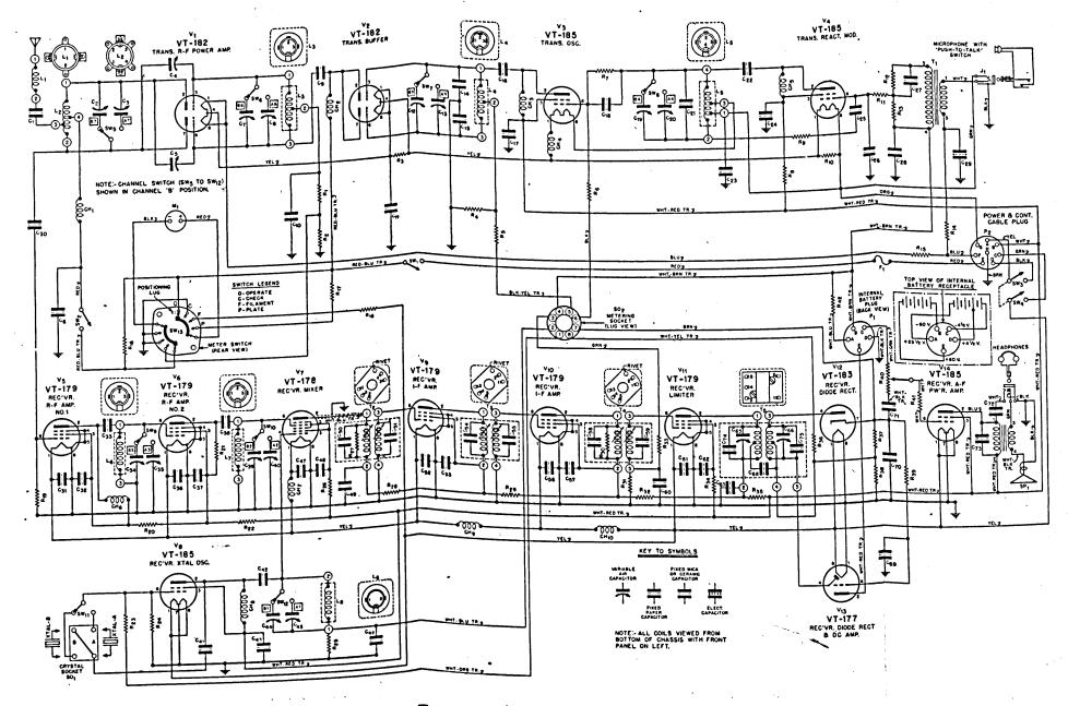
FIGURE 51. BC-659-A Transmitter and Receiver-Schematic Diagram.
