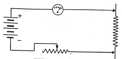
FIGURE 4. Series type ohmmeter.
