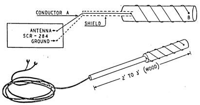
FIGURE 49. Probe type antenna.
