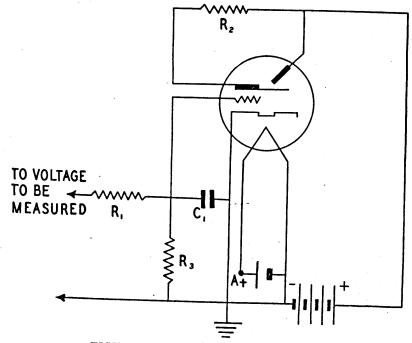
FIGURE 3. Electron-ray tube application.
