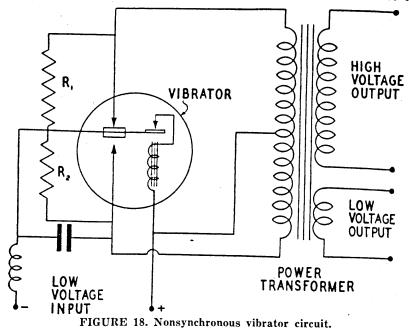
approximately 60 cycles per second. The resulting voltage changes in the primary are stepped up so that high voltage AC is present at the terminals of the high voltage secondary and low voltage AC is present at terminals of the low voltage secondary. A rectifier system must be used to obtain DC voltage for radio equipment from the secondary. Resistors  $R_1$  and  $R_2$  prevent arcing at the vibrator points and may be replaced with suitable
