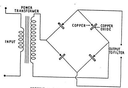
FIGURE 21. Full-wave bridge rectifier.
