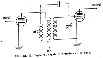
149. CONDENSERS. Replacement condensers must have the same capacity and at least as great working voltage as the part they replace. Electrolytic condensers must never be used where AC voltages may be applied to them. An expedient whereby a 81
