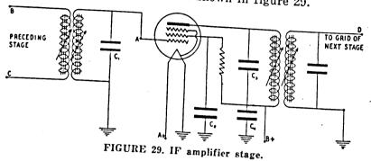
b. Tests. Tests for operation and alignment are similar to those for RF amplifiers. The correct IF signal should be fed to the mixer input (point B and ground of fig. 27) and the RF oscillator should be disabled. To check the band width, note the meter reading at the correct IF, and then shift the frequency of the signal source an amount specified by the manufacturer on each side of the correct IF and repeat the measurement. Readings should be approximately the same as at the correct IF.
