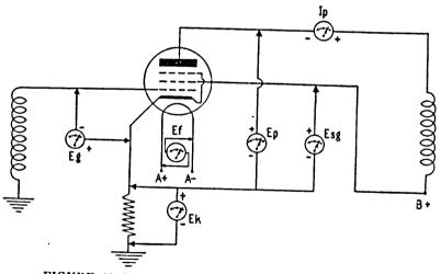
FIGURE 42. Meter connections for checking pentode stage.
