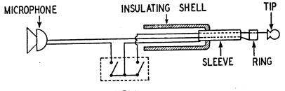
SWITCH FIGURE 13. T-17 Microphone circuit.
