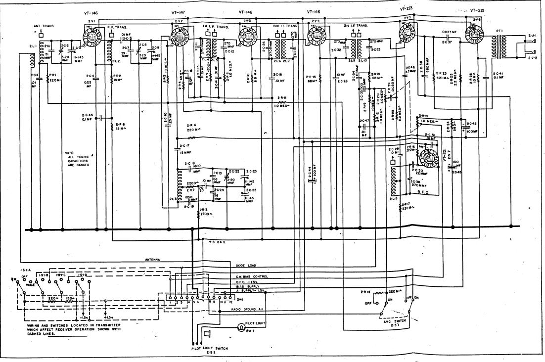
FIGURE 54. BC-654 Receiver-Schematic Diagram. Extract From Fig. 42, TMII-275 RadioManual.EU must include all auxiliary equipment, spare parts and vehicular installations. An historical record of all inspections and all maintenance work should be kept.
