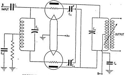
FIGURE 39. Push-pull power amplifier stage.
