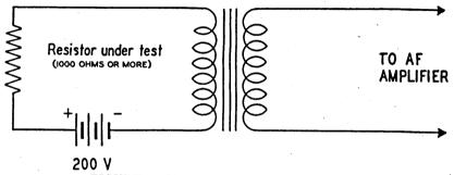
FIGURE 7. Circuit for testing noisy resistors.
