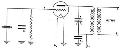
FIGURE 36. Crystal oscillator stage.
