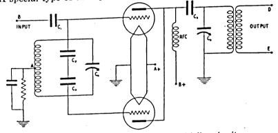
FIGURE 38. Push-push frequency multiplier circuit.
