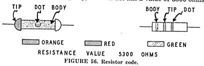
c. Band system. Resistors may also be marked by three colored bands. The band nearest the end of the resistor is the body color, the next band is the tip color, and the third band is the dot color. A fourth band may be added to indicate tolerance as follows:
