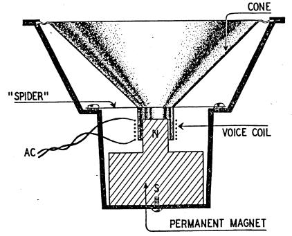
FIGURE 12. Permanent magnet, dynamic speaker.
