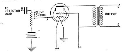
FIGURE 33. AF amplifier stage.
