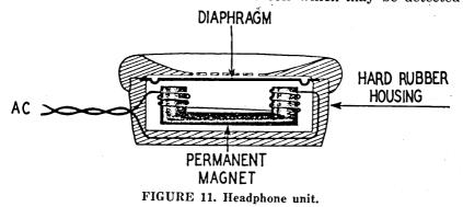
with a continuity tester. The diaphragm may become bent or broken or may be assembled incorrectly. Cords and plugs and electrical connections should be checked.
