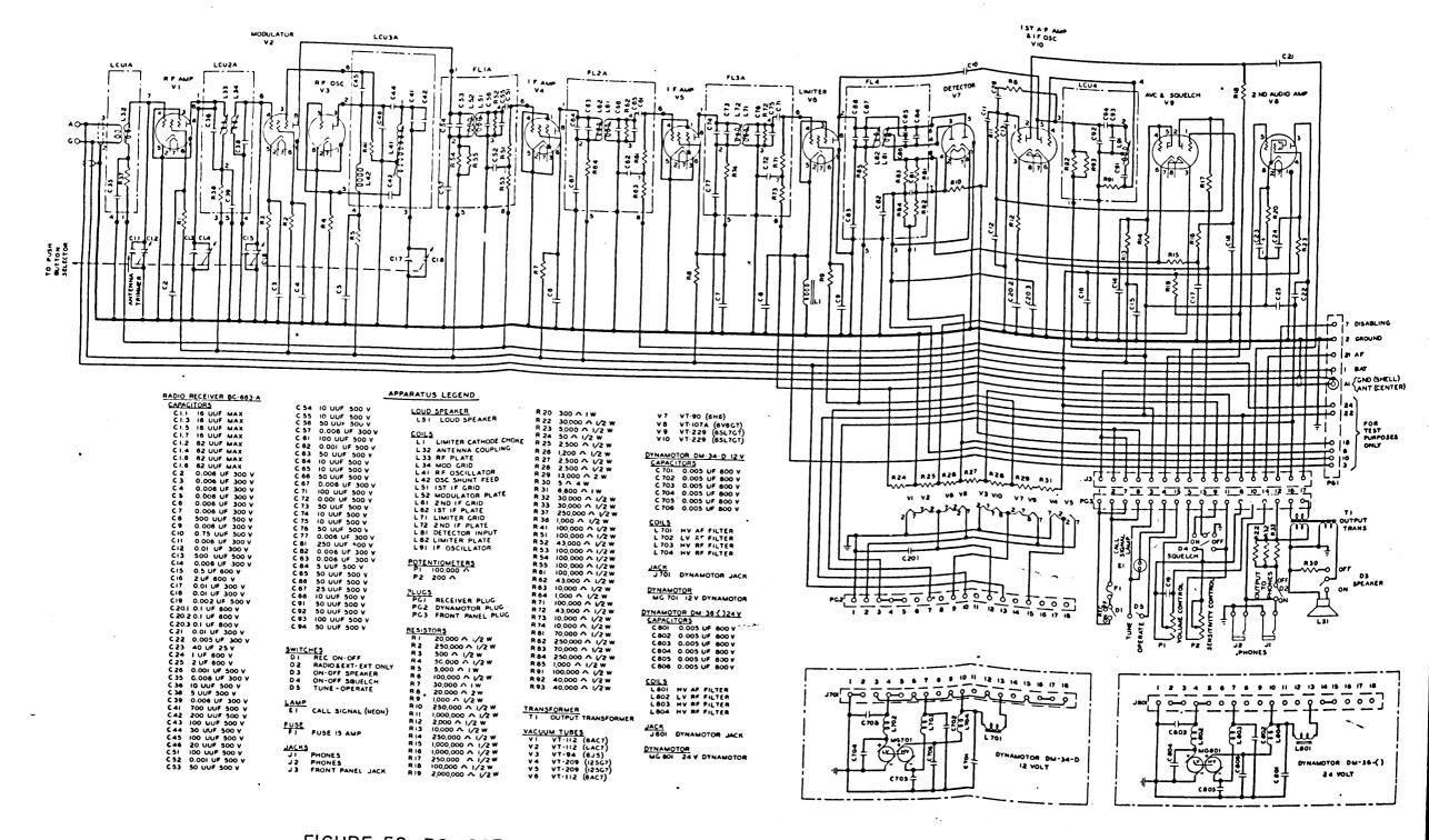
FIGURE 52. BC-683 Receiver-Schematic Diagram. Extract From Fig. 4, TMII-620
