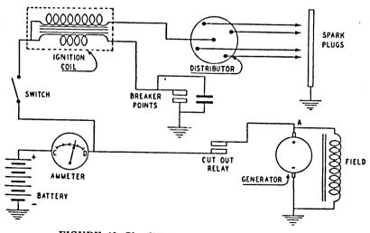
FIGURE 48. Simplified vehicle electrical system.
