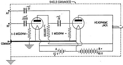
FIGURE 6. Untuned signal tracer.
