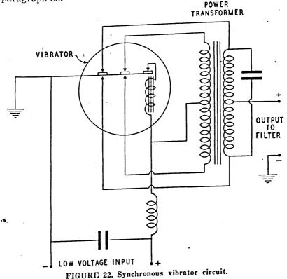
89. SYNCHRONOUS VIBRATOR CIRCUIT. A synchronous vibrator circuit is shown in figure 22. This circuit is similar to figure 18 except that two contacts have been added to the vibrator armature so that a separate rectifier circuit is not required to obtain DC output. Tests are the same as those mentioned in para-
