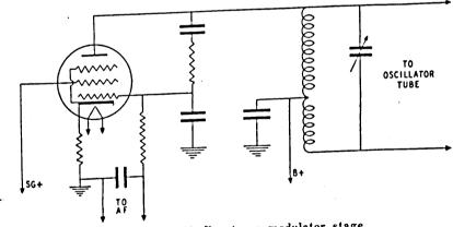
FIGURE 40. Reactance modulator stage.
