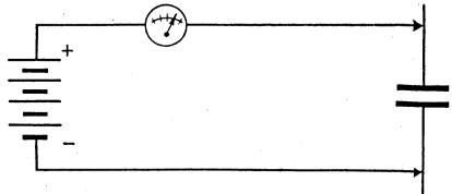
FIGURE 8. Condenser working voltage test.
