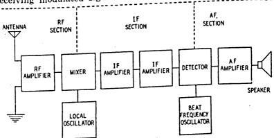
FIGURE 21. Superheterodyne AM receiver block diagram.
