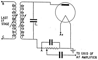
FIGURE 31. Diode detector stage.
