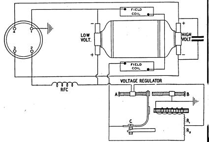
FIGURE 16. Generator circuit.
