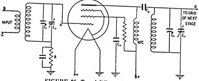
FIGURE 25. Tuned RF amplifier stage.
