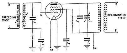
FIGURE 30. Limiter stage.
