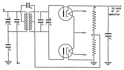
FIGURE 32. Double diode, differential discriminator stage.
