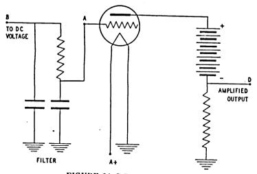
FIGURE 34. DC amplifier stage.
