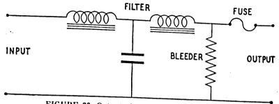
FIGURE 23. Output circuit-vehicle power supply.
