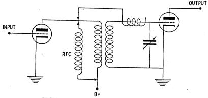
FIGURE 46. Improvised coupling condenser.
