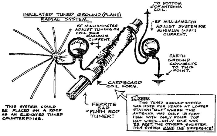
THIS SYSTEM COULD BE PLACED ON A ROOF AS AN ELEVATED TUNED COUNTERPOISE.
