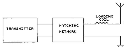
Example: For 175 mmfd antenna capacitance  $L = 4726 \text{ mh}$  at 175 KHz operating frequency.
