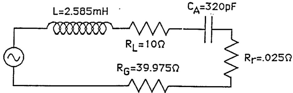
Figure 2. Transmitting loop of a typical 1750m installation.
