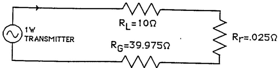
Figure 3. Transmitting loop in resonance reduces to resistances.
