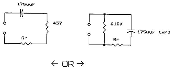
Values for  $R_g = 20$  ohms,  $R_i = 2$  megohms,  $R_e = 500$  ohms
