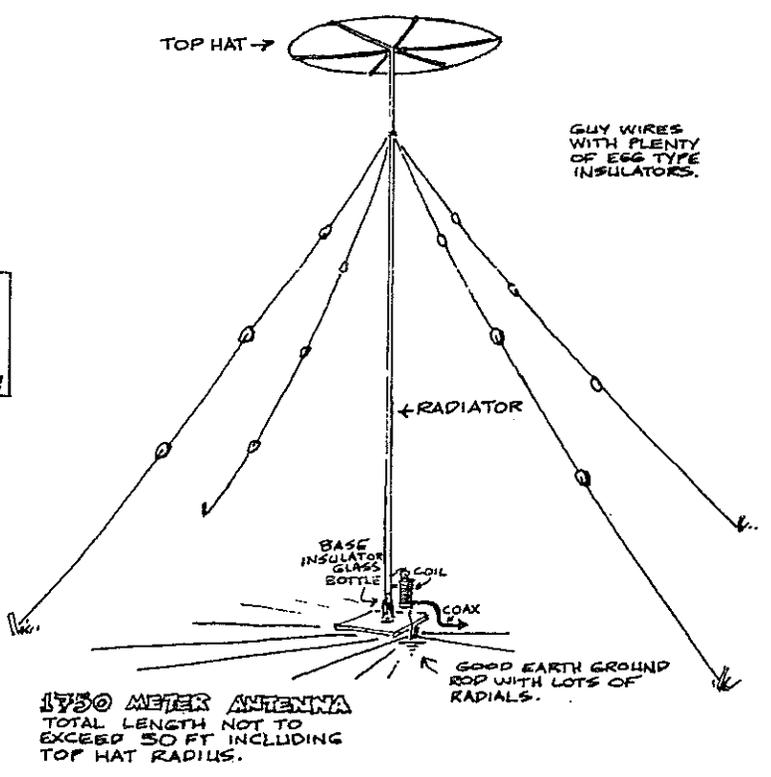
While the the 2,842-ohm capacitive reactance is easily tuned out by a 2,842-ohm inductive reactance, still buried in that 50-ohm resistance is a useful(?) radiation resistance of 0.025 ohms. Graphs showing radiation resistance for electrically short top-loaded verticals are found in various engineering literature (1,2,3,4). Figure 2 shows a schematic representation of the transmitting loop.
