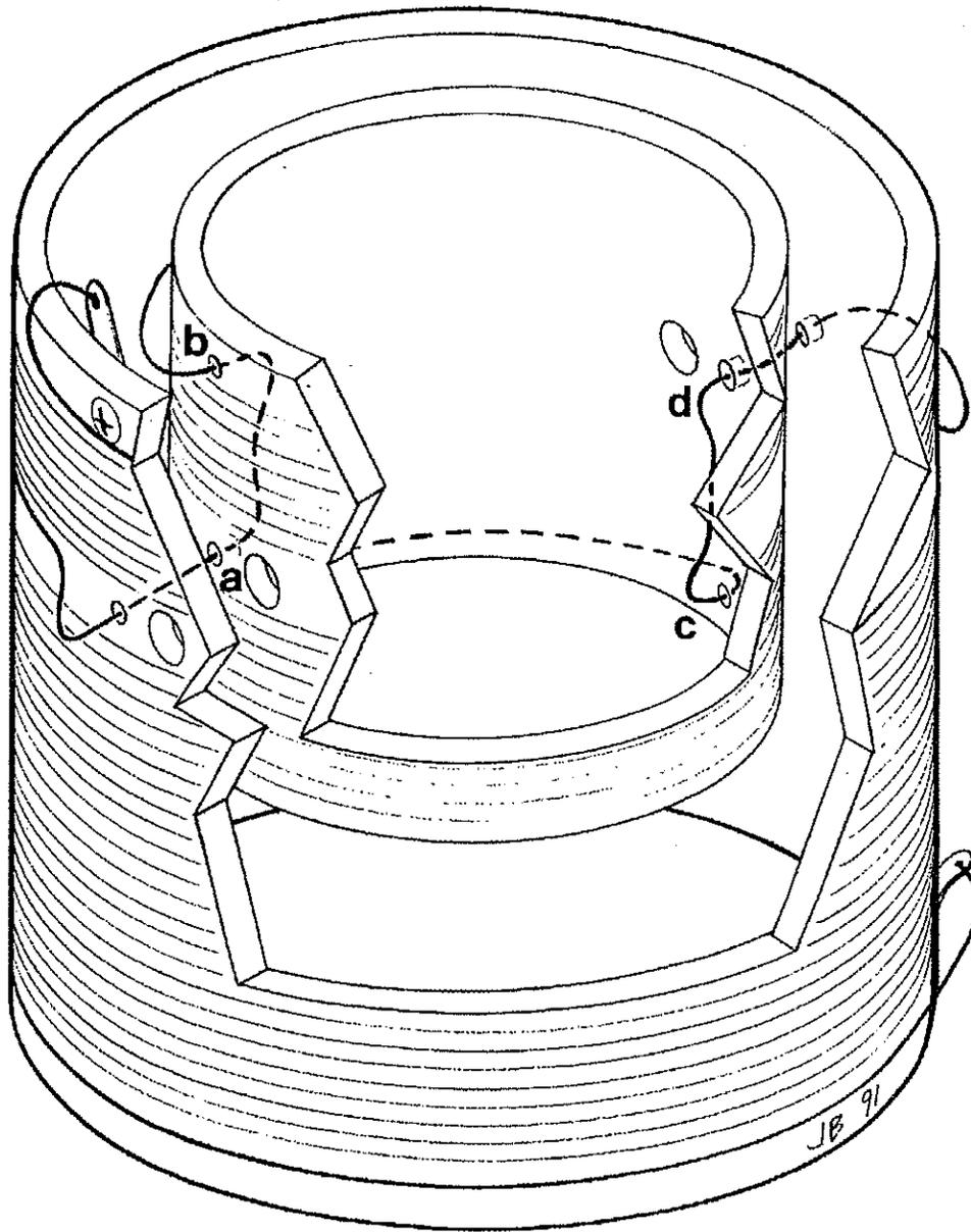
The variometer provides a large inductance range for antenna tuning. Two basic types of variometers exist: one that is tuned by rotating the inside coil and the other by lifting the inside coil in and out. As shown in this illustration, the smaller inside coil rotates to aid or reduce the total inductance.
