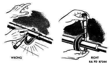
Do not check a part that is moving or rotating. Damage to the micrometer and possible injury to the operator will result.
