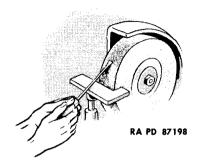
Grind blade of cone-pointed awl to point. Rotate awl during grinding to keep point centered. Be careful that the revolving wheel does not catch the point and cause damage. Dip blade frequently in water or wet grind it. If grinding a flat-pointed or special shaped awl blade, hold blade against abrasive wheel in positions to preserve or restore original shape.
