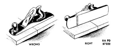
Do not plane with grain of wood sloping down. The wood is likely to tear and jam the plane. Always have grain of wood sloping upward in direction of planing stroke.
