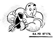
Do not force wheel onto spindle. It must slide on easily with 0.003to 0.005-inch clearance.
