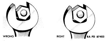
Never turn adjustable wrenches so pulling force is applied to adjustable jaw. Wrench is likely to slip or break. Always turn wrench so force is received by stationary jaw.
