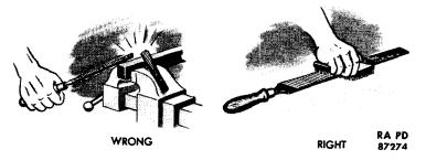
Never use a file without a handle. It is dangerous. Install handle before using file for any job, no matter how small.
