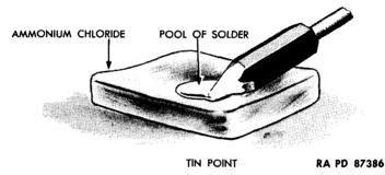
7. Clean tinned point each time it is removed from heater. When pits form on copper back of tinned area, heat copper and dip in water to remove scale.
