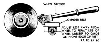
1. Adjust tool rest to permit wheel dresser to contact abrasive wheel on centerline of wheel as illustrated.
