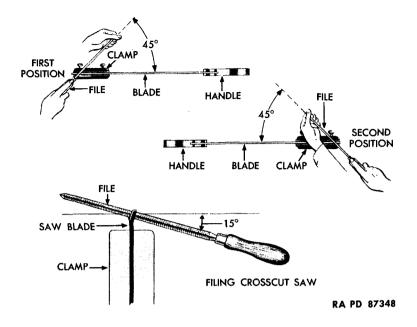
After one side of saw is filed, turn it around and file other side. Never file all teeth from same side, as this causes saw to run to one side.
