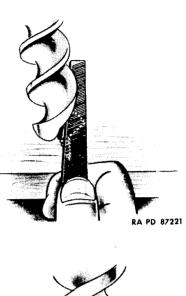
Stop filing when a fine bur appears on cutting edge.
