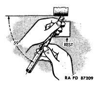
4. Slowly place heel of drill against grinding wheel. Then gradually raise shank end of drill and twist drill in fingers in a counterclockwise direction while grinding wheel approaches the ~utting edge. Exert only enough pressure to grind the drill without overheating. Frequently cool drill in water while grinding.
