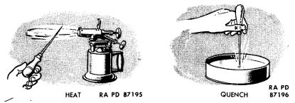
Quickly rub hardened end with aluminum oxide abrasive cloth or oilstone to brighten it. Watch color return to tip from heated portion of blade and quench when light straw color arrives at point. Polish blade with aluminum oxide abrasive cloth and crocus cloth.
