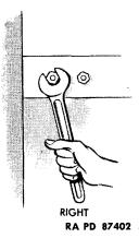
Never use a wrench which fits the nut poorly. This practice batters nuts and spreads wrenches. Use correct size wrench.
