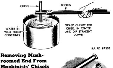
It is dangerous to use a metalcutting chisel with a mushroomed head. Grind head to original shape. Harden chisel after removing mushroom. RA PD 87256
