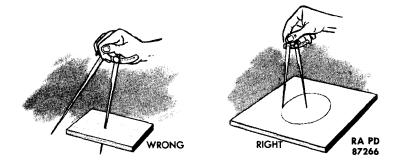
Do not lay dividers on bench when not in use. They may be damaged by other tools. Keep them in case or wrapped in cloth and stored in a safe place.
