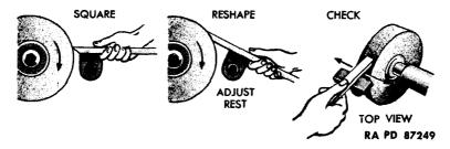
**NOTE:** Special holding fixtures are available. Their use greatly simplifies grinding of chisel type tools.
