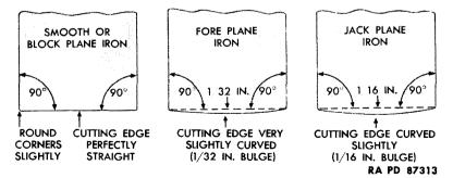
2. Bevel may be straight or slightly concave. It must never be rounded out.
