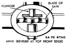
Without Saw Set. Prepare a steel or hardwood block similar to sketch. Dimensions shown are minimum; block may be larger. Angle of the bevel must be determined by examination of the saw to be set; however, angle A must be not less than 146 degrees or saw teeth will break off when set.
