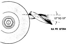
Grind heel to an angle of 12 to 15 degrees (9 degrees for drilling extremely hard material). Failure to provide sufficient clearance is the principal cause of drills splitting up the web.
