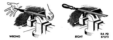
Do not use excessive pressure while filing. This results in clogging file and stripping teeth. Use a long, steady, uniform stroke. Hold handle with right hand. Hold end of file between thumb and first finger of left hand.
