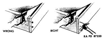
Do not twist off strips of waste with blade. This dulls and bends teeth and may spring blade. Break off strips of waste with hand or mallet.
