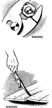
Do not use pliers as a pry bar. Handles may bend or break. Use tools only for purpose for which they are designed.
