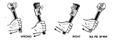
Do not use pipe to increase wrench leverage. Wrench may bend or break. Use longer wrench.
