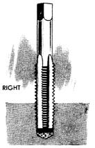
HOLE HAS SUFFICIENT DEPTH TO KEEP CHIPS FROM BINDING RA PD 87392
