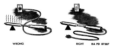
Do not throw coppers into tool box. There is danger of battering the point. Hang coppers up or place on an uncrowned shelf when not in use.
