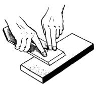
REMOVING WIRE EDGE RA PD 87317
