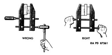
Do not cock clamp to tighten. This procedure may warp, bend, or break clamps. Keep jaws parallel.
