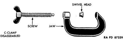
2. Using new parts as needed, turn the screw into position through its boss at end of jaw. Slip swivel head onto ball on end of screw and crimp head sufficiently to hold it on ball.
