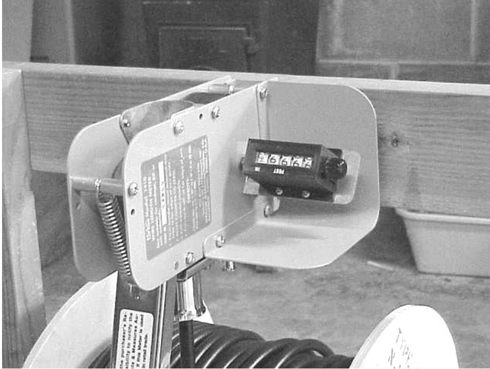
Figure 11 The Hykon 1410 cable meter with a 500 foot roll of RG-213 mounted.
