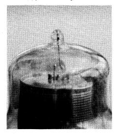
Fig.2A: This type 24A valve has the grid lead broken off flush with the glass sealing tip.
