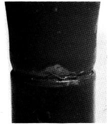
Fig.1A: A common problem with metallising. Not only has the base become loose, but the earthing wire has lost reliable contact with the shielding.
